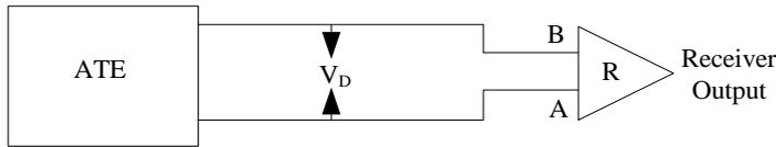
Figure 6. Receiver Propagation Delay Test Circuit
